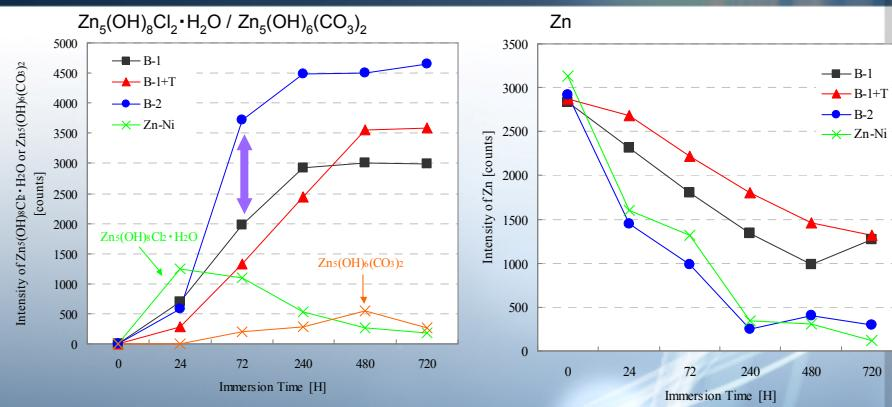
Fig. 4. XRD Intensity Changes of Corrosion Product and Zinc (NaCl Immersion Test)
