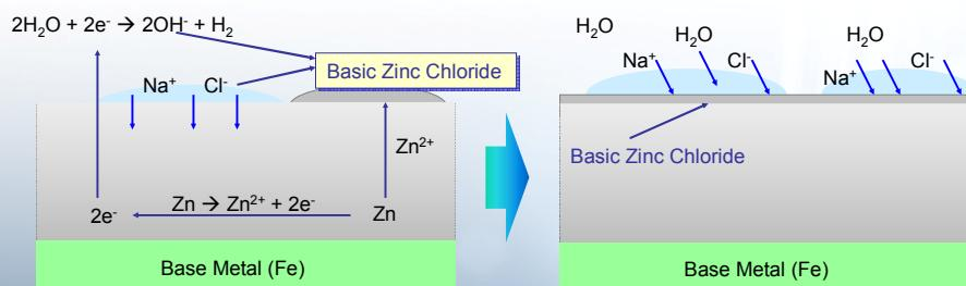
Fig. 11. Corrosion Protection Mechanism of Zn/Al Flake Coating
