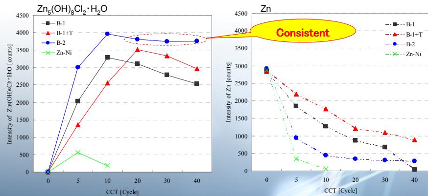
Fig. 6. XRD Intensity Changes of Corrosion Product and Zinc (CCT)
