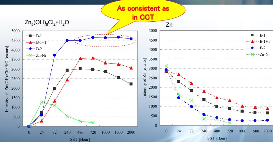
Fig. 8. XRD Intensity Changes of Corrosion Product and Zinc (SST)
