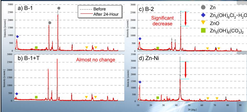
Fig. 2. XRD Pattern of Each Film Before and After 24-Hour NaCl Immersion Test
