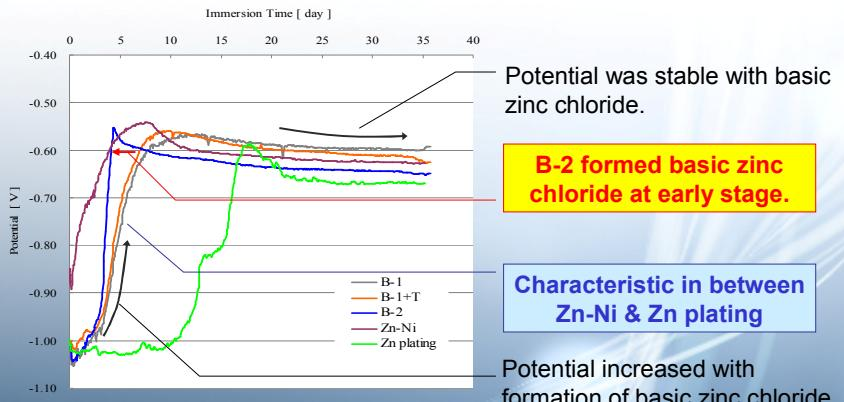
Fig. 10. Time-Dependent Change in Natural Potential of Each Film
