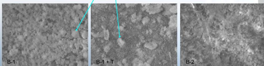
Fig. 9. SEM Image of Each Film After 240-Hour SST
